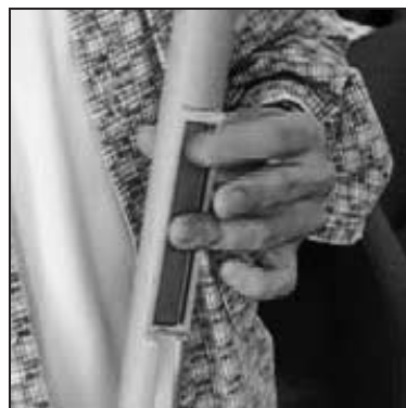
9b. Cloesep of linear potentiometer FSR on The Stick.
