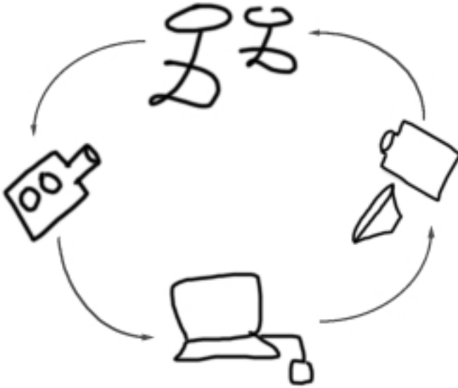
Figure 8. Flow of gesture through a TGarden responsive space: People in a room → {Sensors, Camera} → Computer → {Speakers, Projector} → People in a room.
