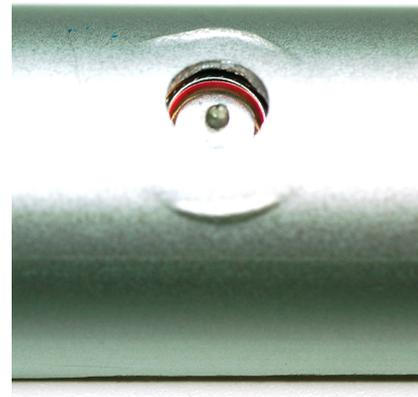
**Figure 3.** Closeup of a tonehole with vibrotactile actuator. The metal ball in the center of the diaphragm is a mass load that lowers the diaphragm's resonant frequency and increases inertia [31].
