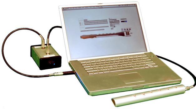
**Figure 2.** The TFD connected to the audio out of a laptop through a current amplifier.
