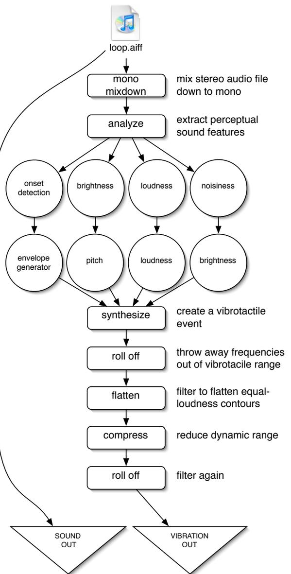
**Figure 5.** Flow chart illustrating audio feature extraction and vibration mapping.
