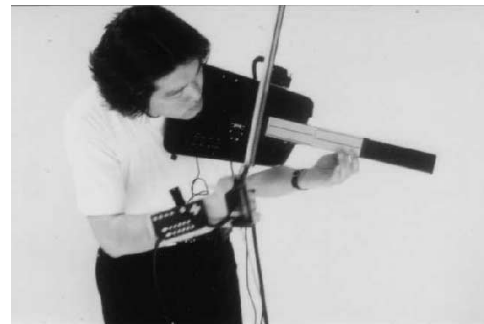
Fig. 3. S. Goto and the SuperPolm, an instrument-inspired controller (violin).
